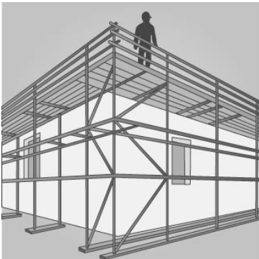
Figure 6: Perimeter scaffold with a fully decked working platform, guardrails and toeboards.
