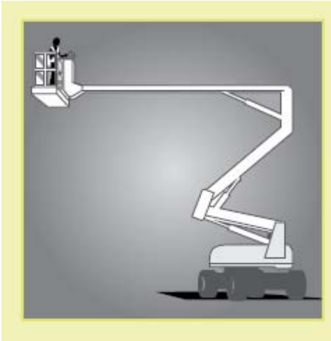
Figure 9: An example of a boom-type elevating work platform. The safety harness and lanyard assembly are not shown for purposes of clarity. The lanyard should be as short as possible and should be attached directly to the designated anchor point on the EWP, not to the handrail.
