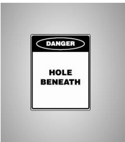
Figure 5: Example of the type of danger sign to be affixed to the hole cover
